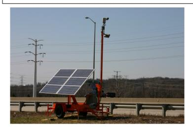
The PEMS-2CT Portable Traffic Monitoring platform provides real-time traffic video and traffic data. The PEMS-2CT uses solar power and wireless communications to provide 24/7/365 autonomous traffic monitoring anywhere in the continental United States. Traffic data and video from the PEMS-2CT can be viewed standalone on a personal computer or integrated into existing traffic management systems.
