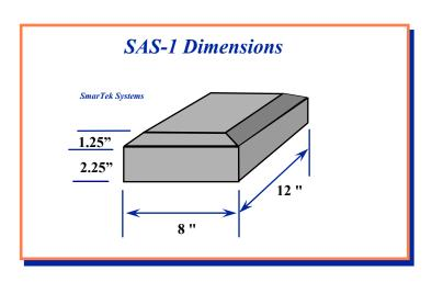
The SAS-1 can monitor 5 lanes and provides for several different interfaces depending on the communication link and the cabinet controller interface desired. The standard SAS-1 output message provides per lane traffic flow measurements of vehicle volume, lane occupancy, and average speed for a selectable update period (1 to 220 seconds). A bit serial vehicle presence relay message or opto-isolated dry contact vehicle presence relay signals (using the SAS Relay Interface) can be provided.
