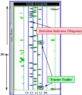
Each "Blob" Shows Position and Strength of Each Vehicle's Acoustic Intensity:
